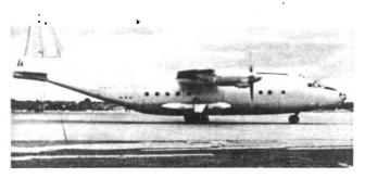
Figure 6-62. An-12 CUB. The standard troop carrier for airborne operations, the CUB has rear-loading ramp for equipment and vehicles. The rear-gunner's turret is a distinctive feature of this aircraft.
